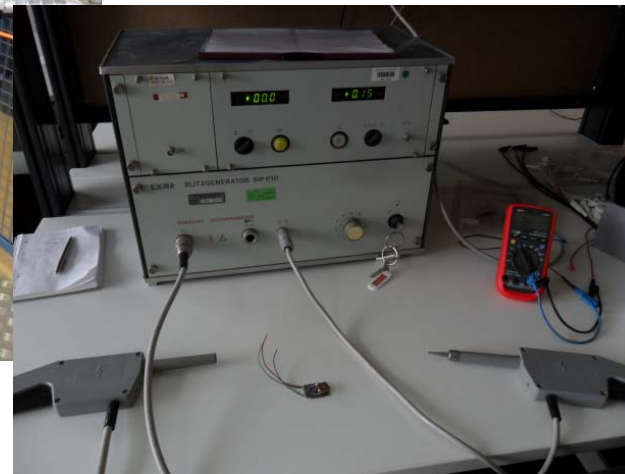
Lightning surge generator (Test robustness of RF components)
